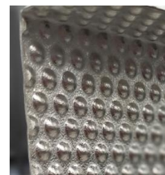
Example of stainless steel embossed structure
