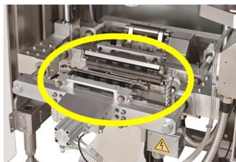
Heating pressure bar with knife of packaging machine (with PTFE Coating)
