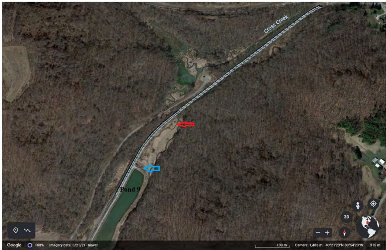
Image 2. Aerial image of Pond 9 leading to Outfall 009. In 2020, Outfall 009 was moved from the location at the blue arrow at the end of the discharge pipe to the location at the red arrow prior to merging with Cross Creek in order to prevent TDS.
