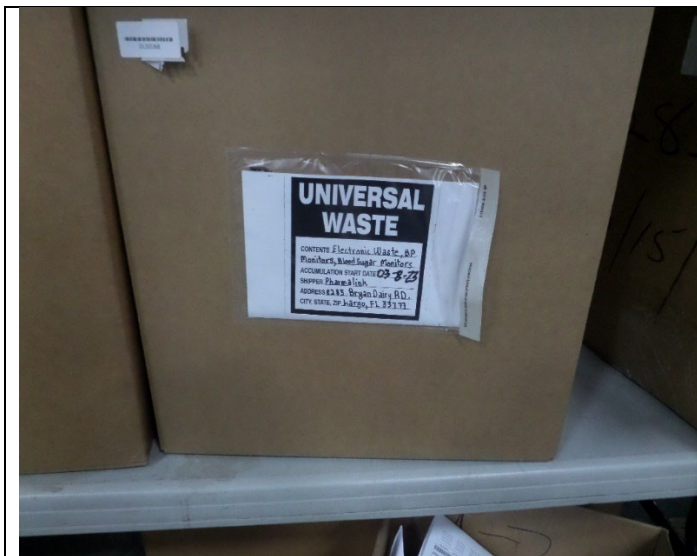
Batch Packing Area. Refractory Area. The inspectors observed the universal waste container was not marked with a date The facility marked the container with the date March 8, 2023. Photograph 11 taken at 12:52 p.m.
