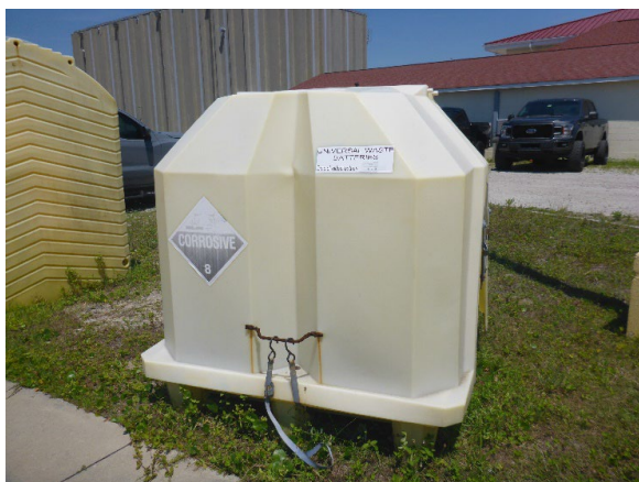
Photo 5: Closed container labeled universal waste batteries.
