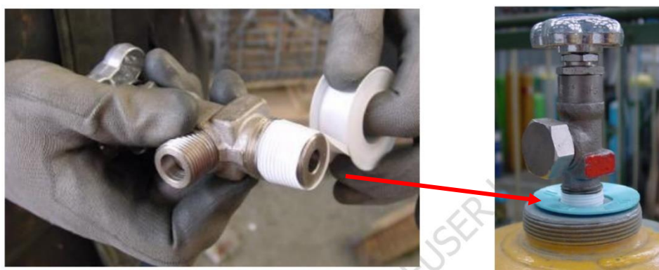
Figure 10: example of a joint with PTFE.
