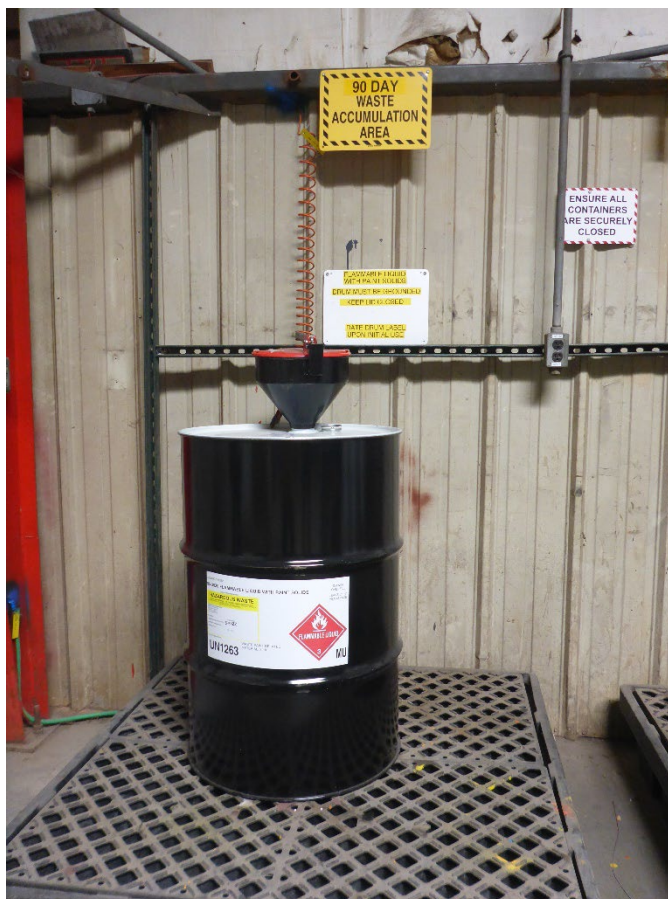
Photo 6: One 55-gallon drum of waste paint related material on a secondary pallet in the CAA. The drum was closed with a latched funnel lid, and it was labeled D001 / D035 hazardous waste flammable liquid with paint solids. Although the drum was identified with a DOT flammable liquid hazard placard, it was not marked to indicate that its contents are also toxic.
