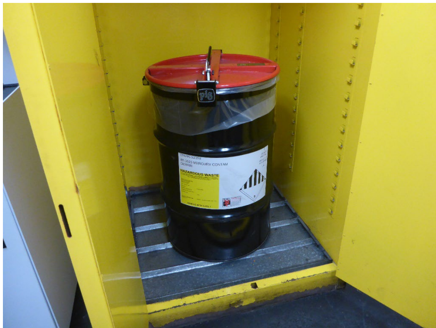
Photo 1: One 30-gallon drum observed in the SAA for managing D009 hazardous waste mercury contaminated debris generated in the Mercury Laboratory. The drum was labeled as hazardous waste and closed with a latched lid. Although the fire cabinet was marked to indicate that its contents are toxic the hazardous waste container was not marked with an indication of the hazards of its contents.
