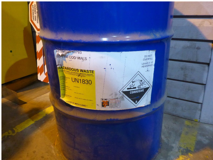
Photo 3: One 55-gallon drum observed in the SAA for managing D002 / D007 / D009 / D011 hazardous waste sulfuric acid solution generated in the Wastewater Treatment Laboratory. The drum was closed, and it was labeled as hazardous waste. Although the drum was marked with a DOT corrosive hazard placard, it was not marked with an indication that the contents are also toxic.
