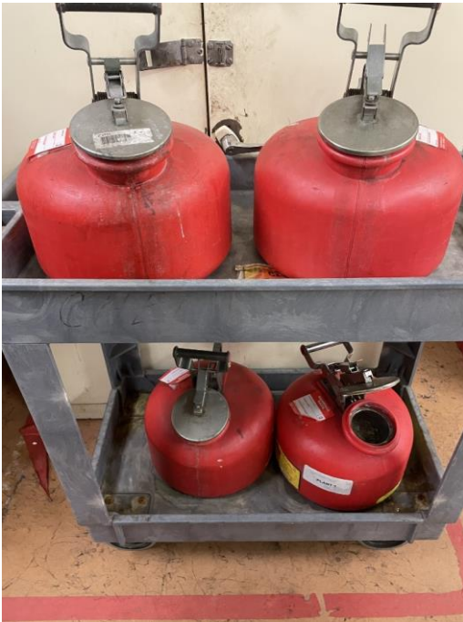
Photograph #1 – Four 2.5-gallon containers of flammable waste and open container.
