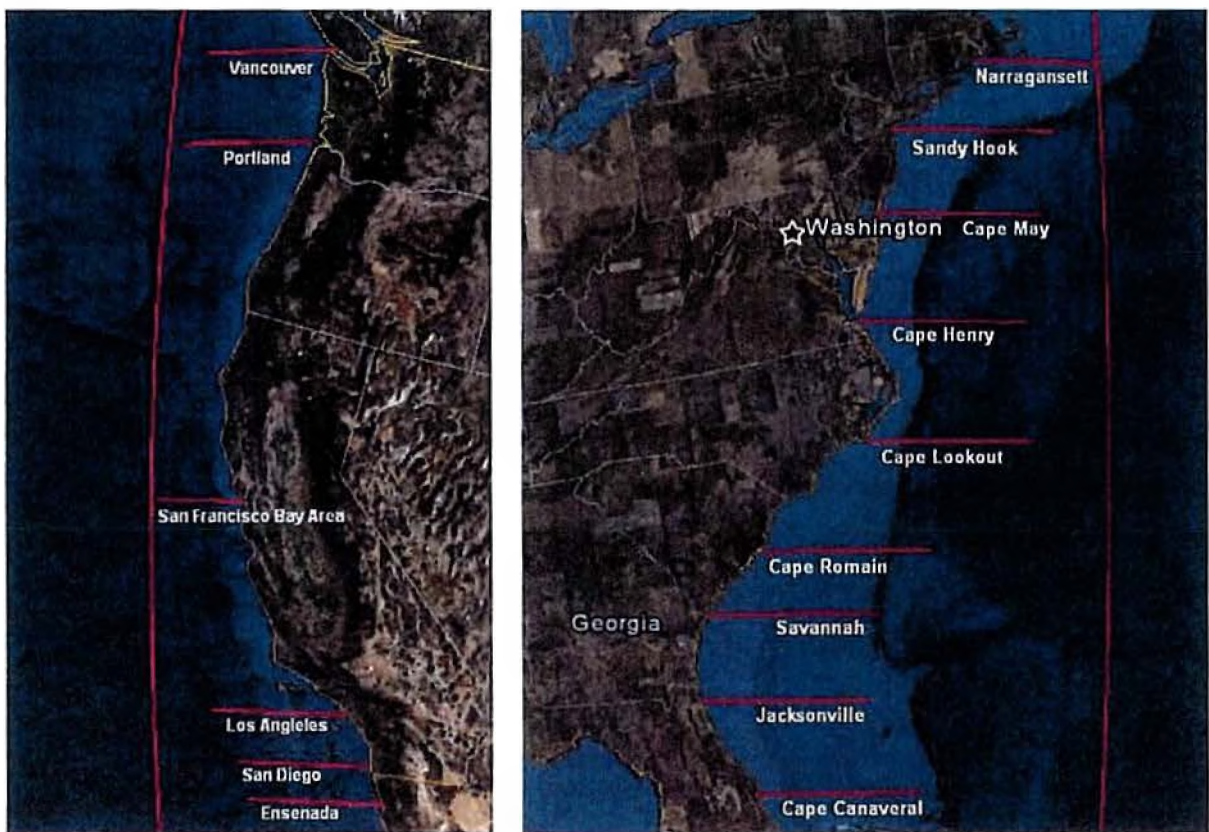
Figure 3. Modeled Source Lines. 21 Emission sources (i.e., the ship) were placed at 40 km intervals along each of the red east-west lines extending from each port)
