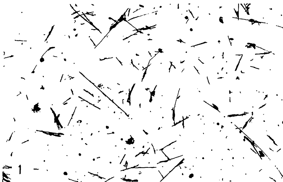
FIG. 1. Suspension of short chrysotile fibers dispersed with Dounce ball tube. \times 5460 .
