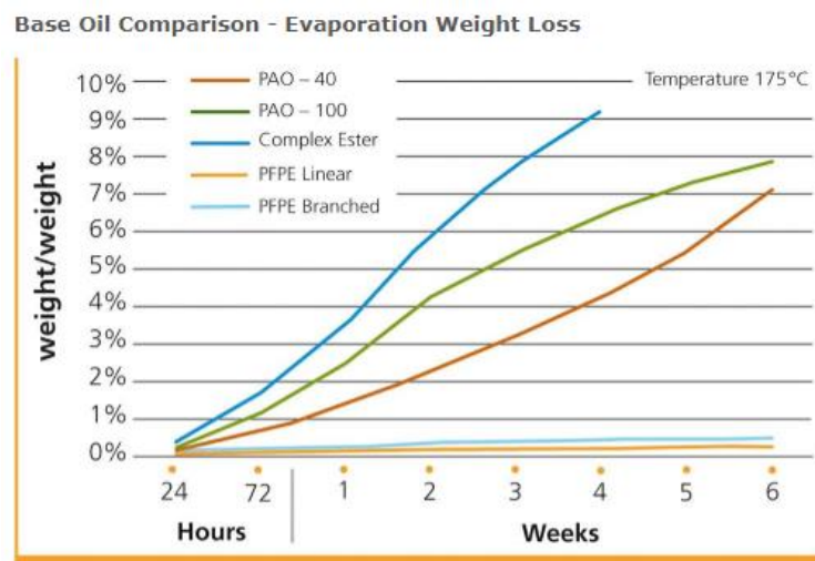
Figure 2 : Base oil evaporation comparison [5]
