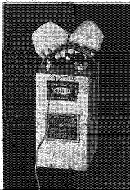
Up with the rack bar and then down, hard. The electric current generator fires the shot. This shows the No. 2 du Pont blasting machine
