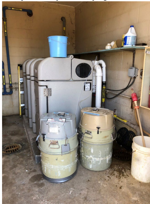
Photo #2. ISCO automatic composite samplers were programmed to collect effluent samples.
