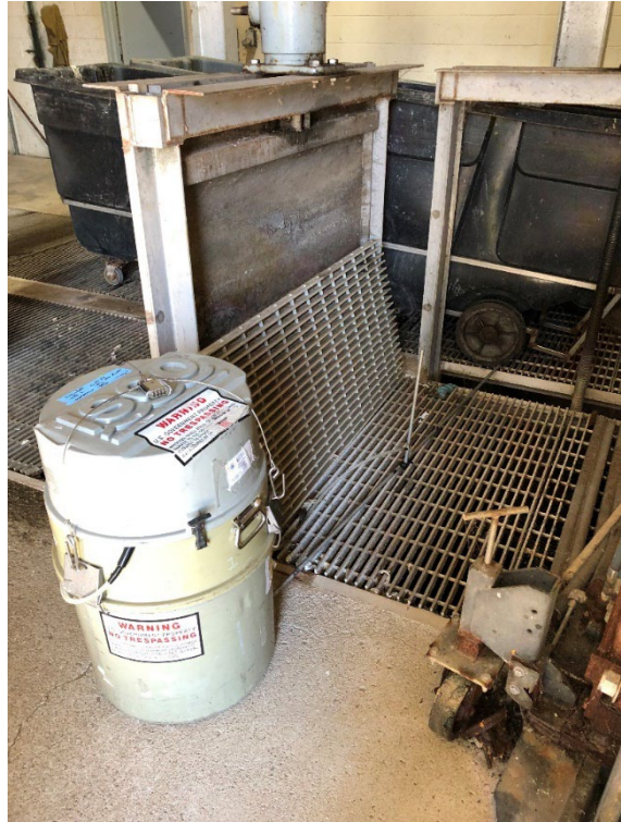
Photo #1. An ISCO automatic composite sampler was programmed to collect influent samples.
