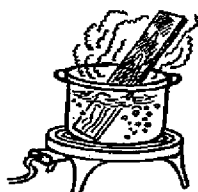
Immersion in boiling water for 1/2 hour produces no more than moderate whitening and recovery is complete in 1/2 hour.
