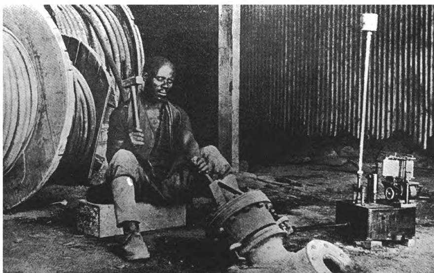
This apparatus is an ergometer set up in the City Deep mine in 1919 in the course of experimental research on heat trauma among mineworkers on the Rand. The machine was designed to record the expenditure of energy and effort by a 'hammer boy', a worker employed in those days in hand drilling. This machine had to be constructed to stand the force of some 14 000 hammer blows during the daily working period.
