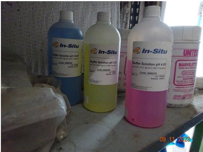
Photograph #15 (DSC03556) Description: pH probe calibration reagents that were expired at the time of the inspection.
