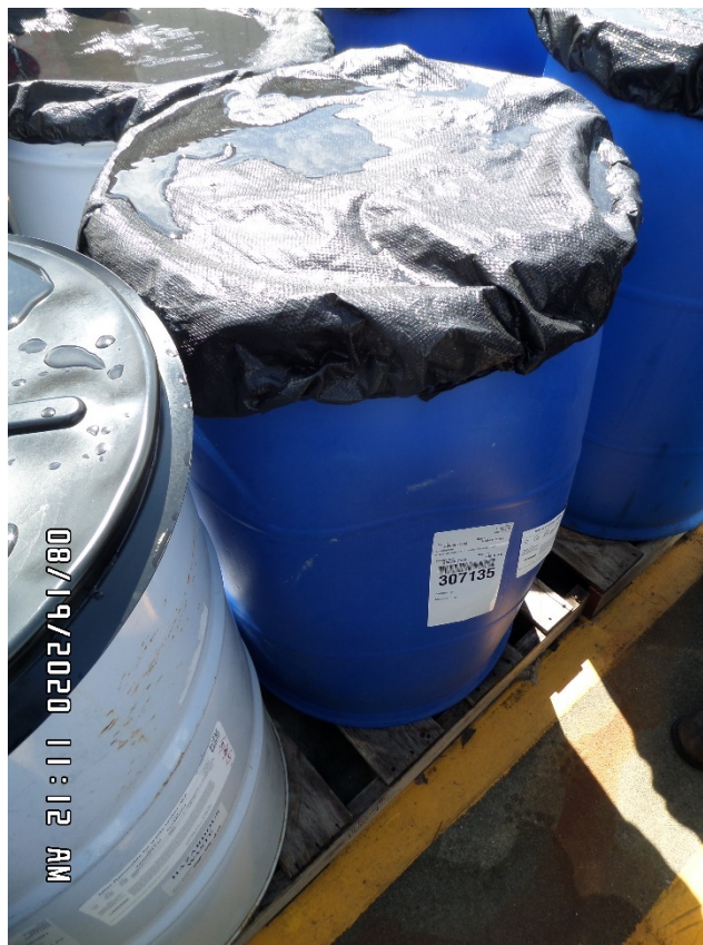
Figure 3 - 55-gallon drum deformed, not labeled dated
