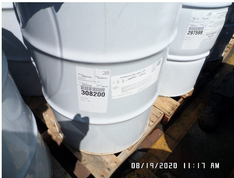
Figure 4 - 55-gallon drum not labeled, missing hazard identification
