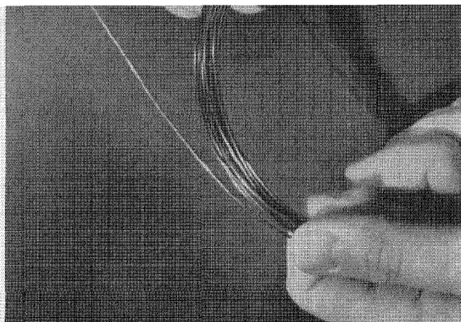
Flexible urethane coating is being used as wire enamel. And the wire can be soldered without stripping away the insulation.
