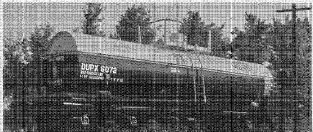
First tank cars with tough urethane coating are now riding the nation's railroads. Easy-to-clean coat has been used on tank trucks.
