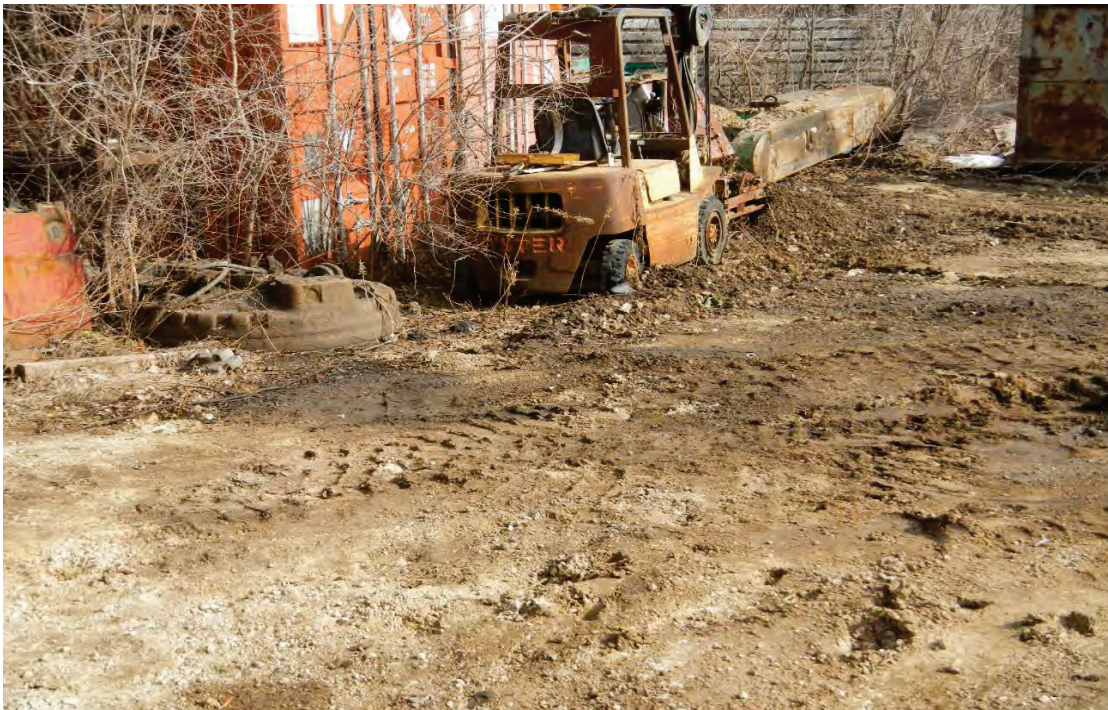
Photo 21, Evidence of significant ground discoloration.
