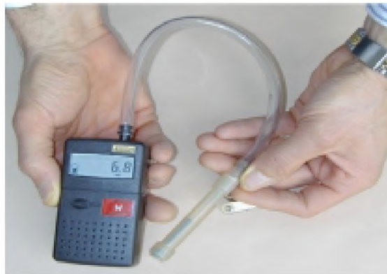
Figure 2.2a: Respirable dust dosimeter (RDD) showing sampling pump and dust tube (Source: Volkwein et al., 2000)
