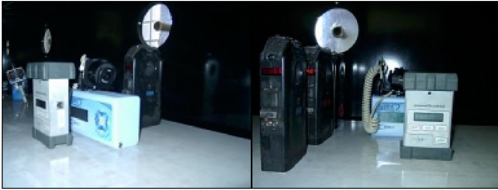
Figure 3.3.4a: Split-2, PDR and Hund dust monitors in the test chamber
