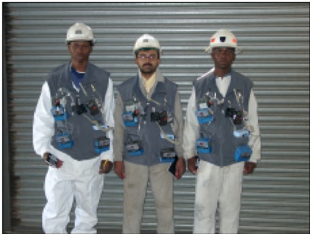
Figure 4.2a: Underground team wearing six personal dust monitors
