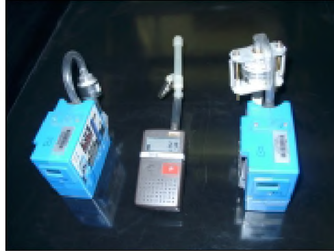
Figure 3.3.1d: Dorr-Oliver cyclone (right), SA cyclone (left) and NIOSH RDD sampler
