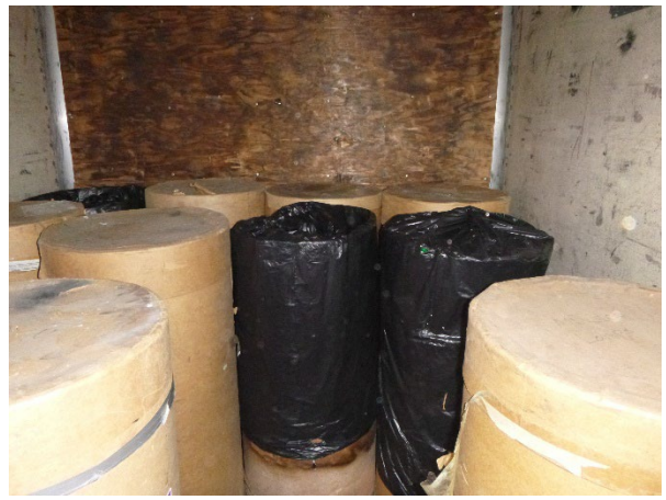
Photograph 20: Trailer storing universal waste lamps in open containers.
