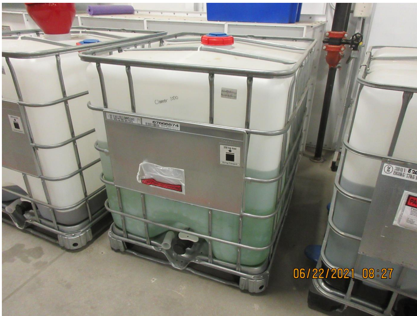
Photo 2 – Tote of spent chemical conversion coating solution (on right) and tote of nonhazardous cleaning solution (center).
