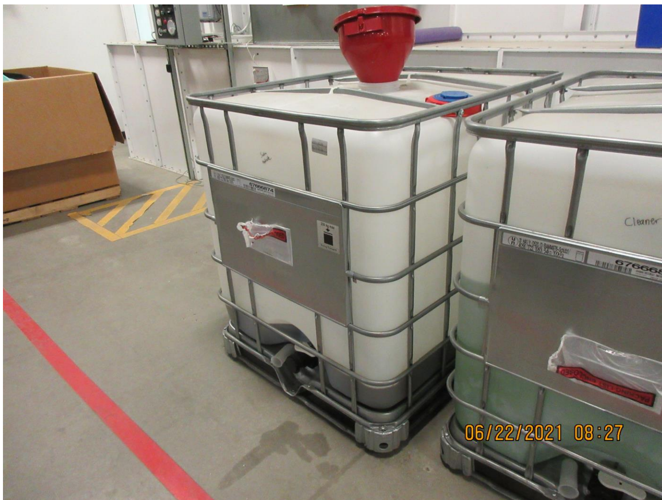
Photo 3 – Tote of spent sodium hydroxide passivation solution (on left) and tote of nonhazardous cleaning solution (on right).
