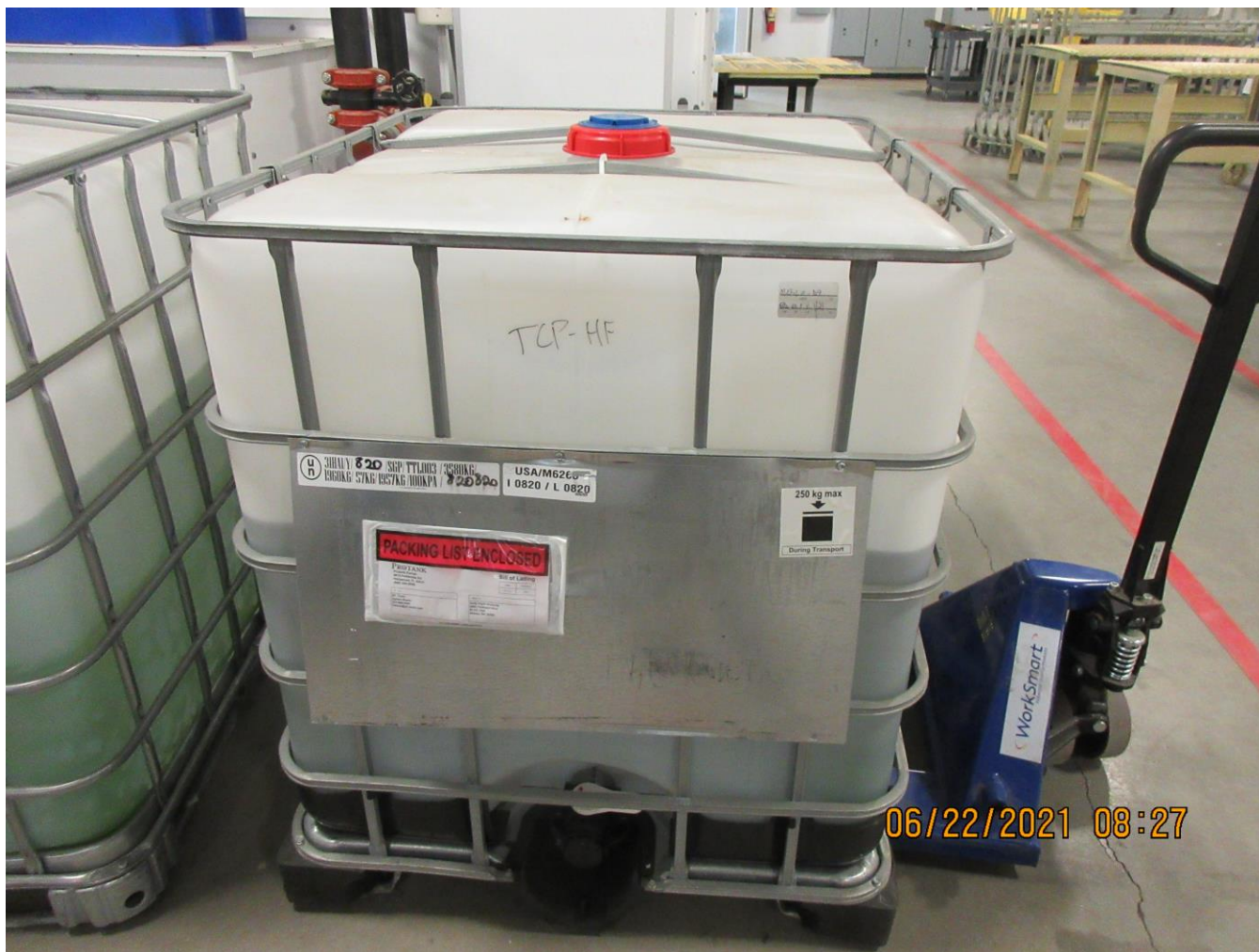
Photo 1 – Tote of spent chemical conversion coating solution.
