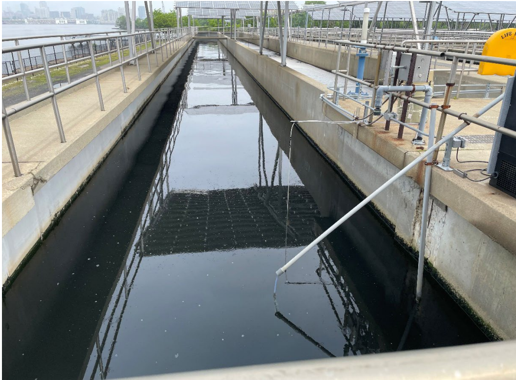
Photo #1. An ISCO composite sampler was set-up in the Northside Chlorine Contact Channel.
