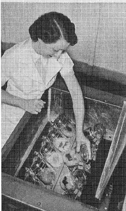
At the Philadelphia Branch Office Laboratory, swatches of cotton material dyed with vat colors are being tested in this Launder-Ometer for fastness to washing.
