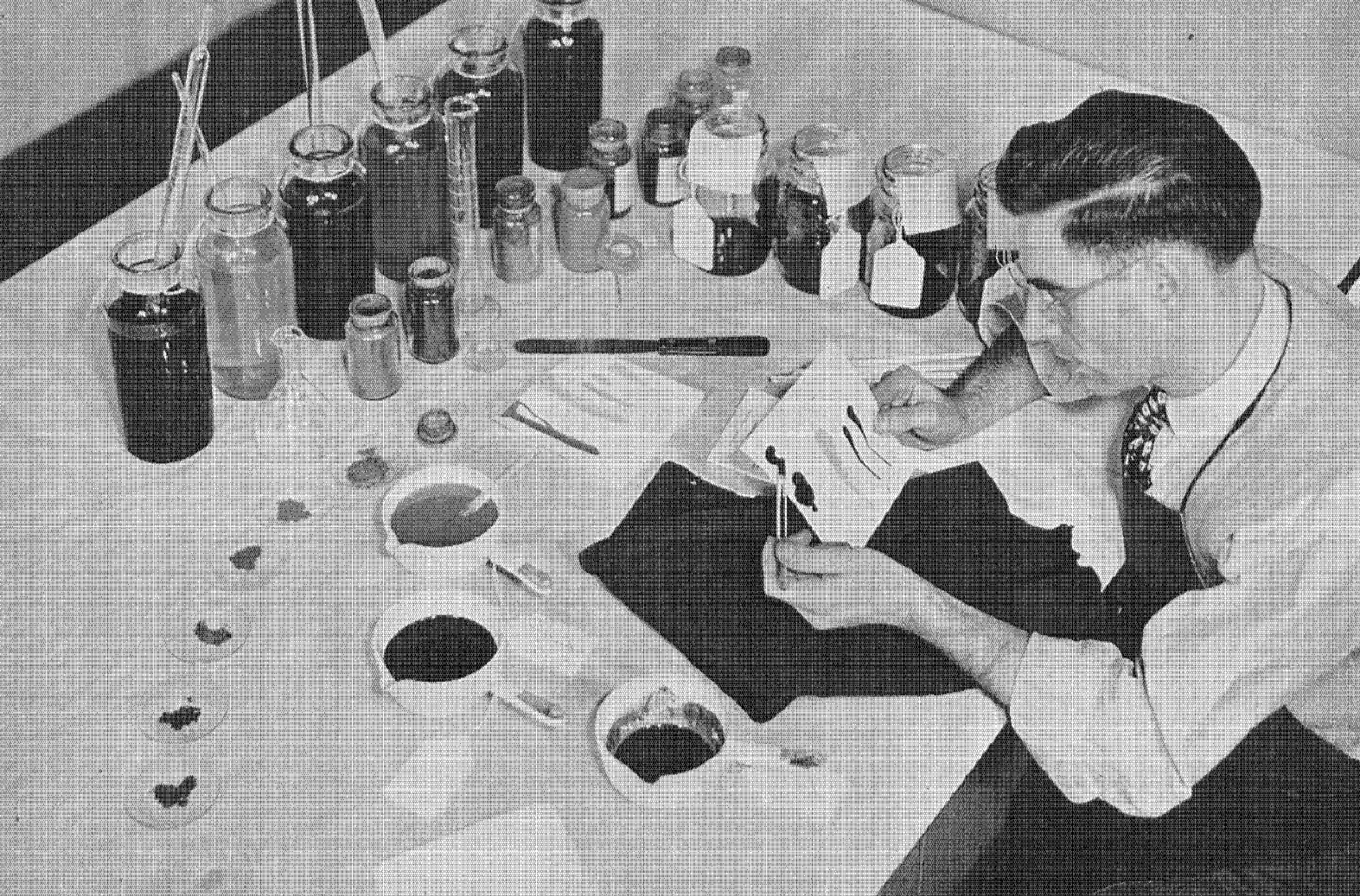
Eight different dyes must be combined to duplicate a shade for a leather customer.
