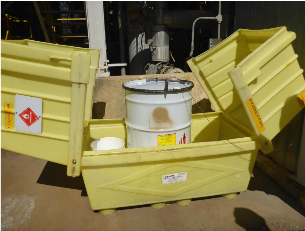
Photo 19: One 55-gallon drum inside a locked, plastic clam-shell secondary containment unit at SAA #17, which is used to accumulate hazardous waste filters that are generated by the CUNO solvent recovery process. The clam-shell was labeled as SAA #17 and marked with a flammable liquid DOT hazard placard. The drum was labeled hazardous waste CUNO filters with IPOH and identified with a flammable solid DOT hazard placard.
