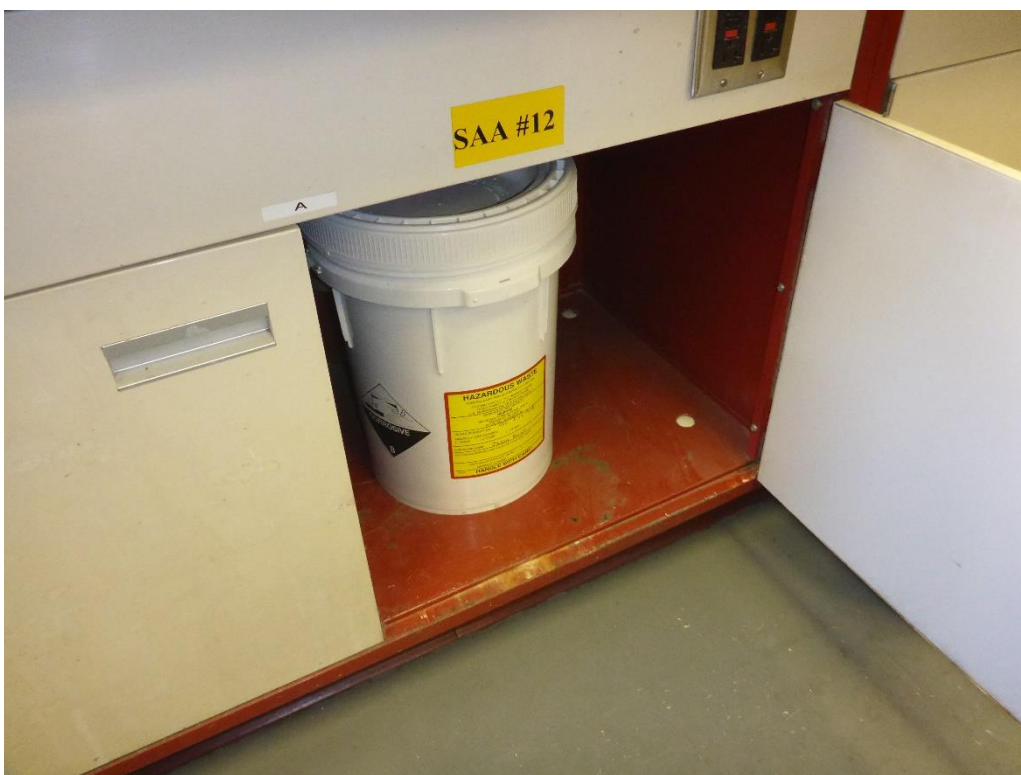
Photo 13: One 5-gallon bucket at SAA #12, which is used to accumulate hazardous waste laboratory chemicals that are generated in the laboratory. The bucket was labeled as SAA #12 and hazardous waste lab pack and identified with a corrosive DOT hazard placard.
