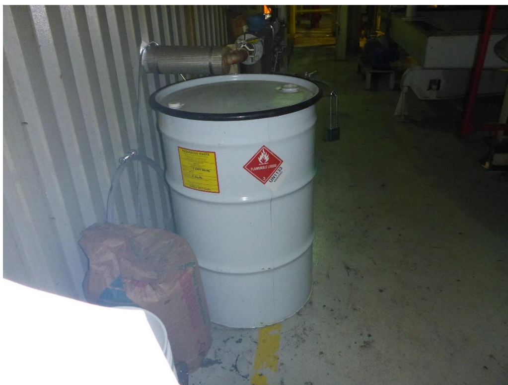
Photo 18: One 55-gallon drum at SAA #16, which is used to accumulate hazardous waste flammable liquids that are generated by sampling and cleaning operations at the C-6424 process. The drum was labeled hazardous waste C-6424 waste and identified with a flammable liquid DOT hazard placard.
