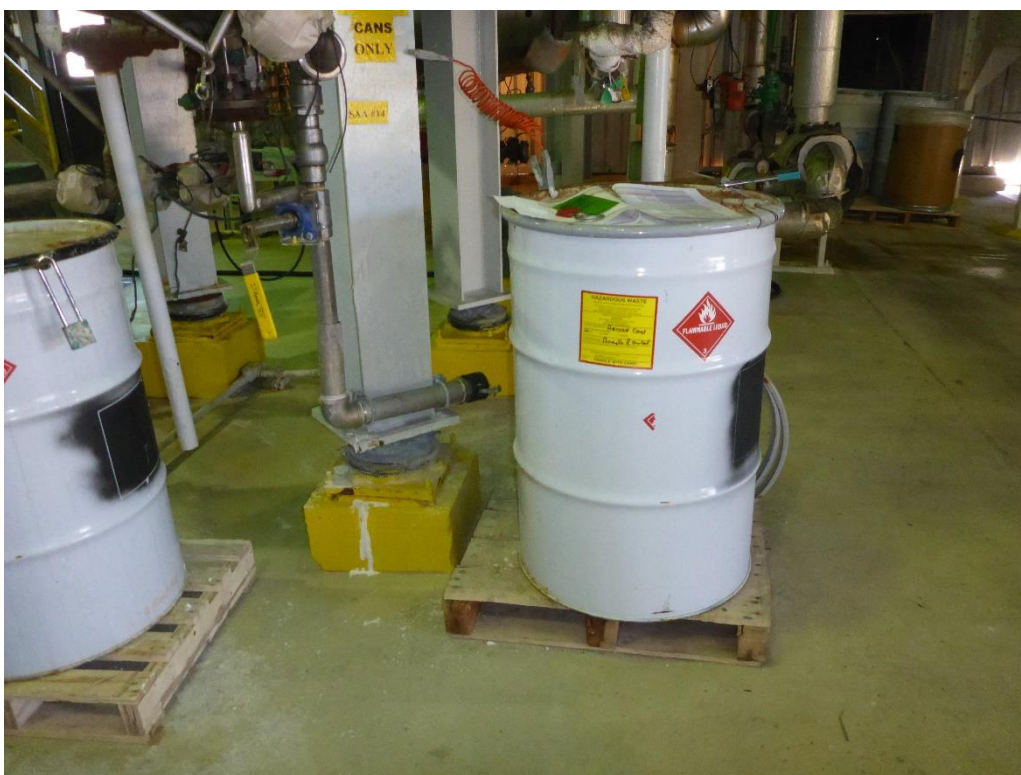
Photo 16: One 55-gallon drum at SAA #14, which is used to accumulate hazardous waste aerosol cans that are generated on this side of the facility. The drum was labeled hazardous waste aerosol cans and identified with a flammable liquid DOT hazard placard.
