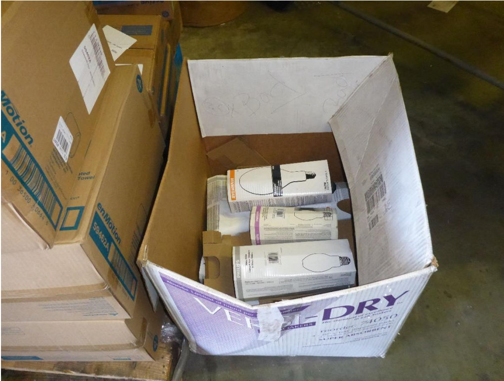
Photo 22: One open, square cardboard box of universal waste metal halide lamps. The box was not labeled “universal waste lamps” or marked with an accumulation start date.
