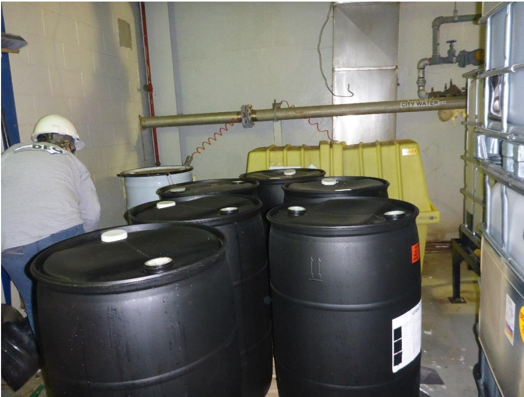
Photo 4: SAAs #4 and #5 located in the Sulfonating Production Area. The locked, plastic clam-shell secondary containment unit is SAA #4, and the secondary containment pallet next to the clam-shell is SAA #5. Nouryon accumulates hazardous waste sulfonating waste that is generated by sampling the sulfonating process in SAA #4, and accumulates hazardous waste sulfonating filters that are generated by the Sulfonating process in SAA #5. The clam-shell was identified as SAA #4, labeled hazardous waste and marked with flammable liquid, toxic and corrosive DOT hazard placards. The drum in SAA #5 was labeled hazardous waste SPS filter bags and products and identified with flammable solid and toxic DOT hazard placard.
