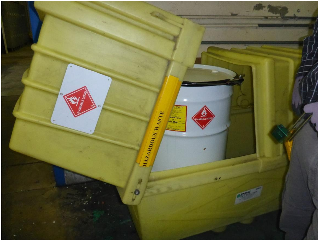
Photo 3: One 55-gallon drum inside a locked, plastic clam-shell secondary containment unit at SAA #3, which is used to accumulate hazardous waste aerosol cans that are generated on this side of the facility. The clam-shell was identified as SAA #3, labeled as hazardous waste and marked with a flammable liquid DOT hazard placard. The drum was labeled hazardous waste flammable liquid and identified with a flammable liquid DOT hazard placard.
