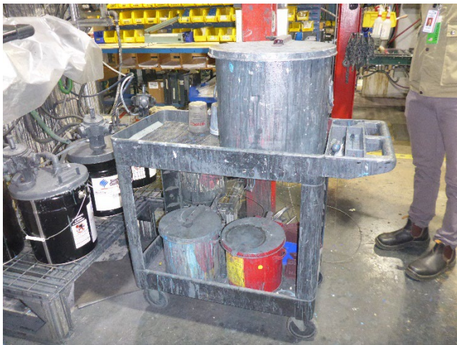
Photo 3: Three containers (two 5-gallon containers and one 10-gallon container) on a mobile cart next to the elevated platform. Each container is holding solvent liquids used to clean dirty paint guns and covers. One container is identified with a hazardous waste label.
