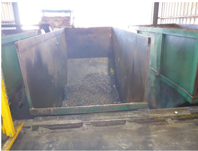
Photo 14: The middle one of three large hoppers just off the edge of the loading dock floor in the Chip Dock. This hopper is in use to accumulate and store metal chips and shavings that do not contain brass.
