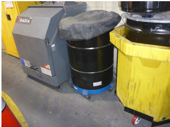
Photo 8: One 55-gallon container in an SAA next to the Flow Line Paint Booth for accumulating hazardous waste solids generated in and around this area. This container was not labeled with the words “hazardous waste,” and it was not marked with an indication of the hazards of its contents.
