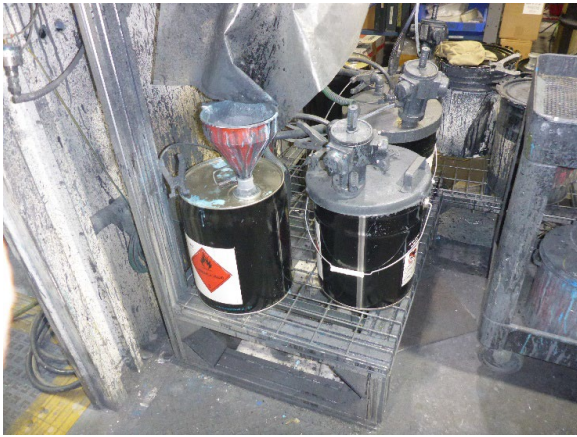
Photo 4: One 5-gallon container in an SAA next to the Main Paint Booth for accumulating waste paint related material generated in and around this area. This container is shown on the left side of the photo on an elevated platform next to four 5-gallon containers of product materials. The container is equipped with an open funnel; it is identified with a flammable liquid DOT hazard placard; it is not labeled with the words “hazardous waste;” and it is not marked with an indication that the contents are toxic.
