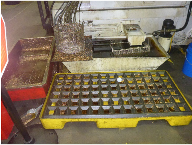
Photo 1: Manufacturing units use either water or oil as a cutting fluid, and each unit is equipped with a reservoir that recirculates the cutting fluids through the manufacturing unit. The process generates scrap metal chips or shavings which are accumulated in a straining basket at each unit.
