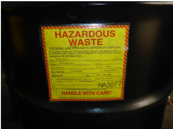
Photo 21: One of two labels identifying the contents of two 55-gallon drums in the CAA as D007, D035, F005 hazardous waste solid paint filters and rags containing methyl ethyl ketone and chromium. The containers were not marked with an accumulation start date.
