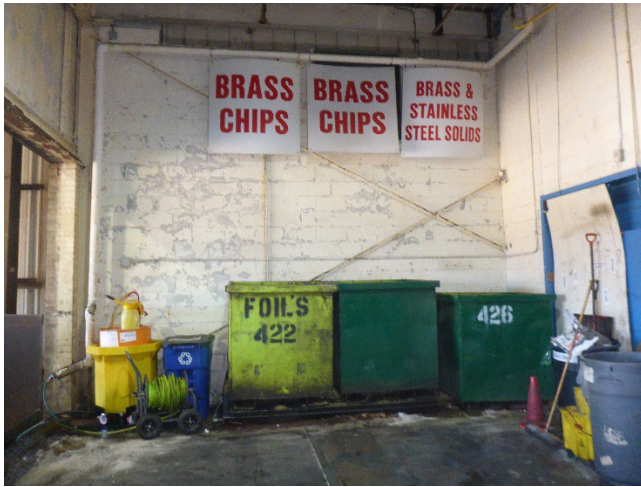
Photo 13: Three bins along the wall at the far end of the Chip Dock. Signs on the wall identify two bins for storing brass chips and the third for storing brass and stainless-steel solids. Cutting fluids drain from these bins onto a secondary containment tray that is connected through a pipe into the 2,500-gallon metal fabricated storage tank.
