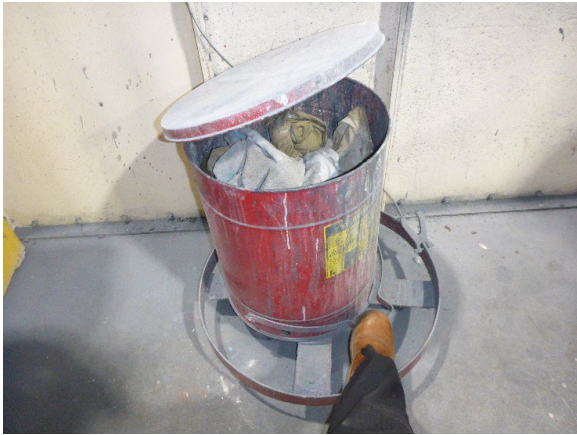
Photo 5: One 20-gallon container in an SAA next to the Main Paint Booth for accumulating hazardous waste solids generated in and around this area. This container, which was observed in the corner just outside of the Main Paint Booth, was not labeled with the words “hazardous waste” and it was not marked with an indication of the hazards of its contents.
