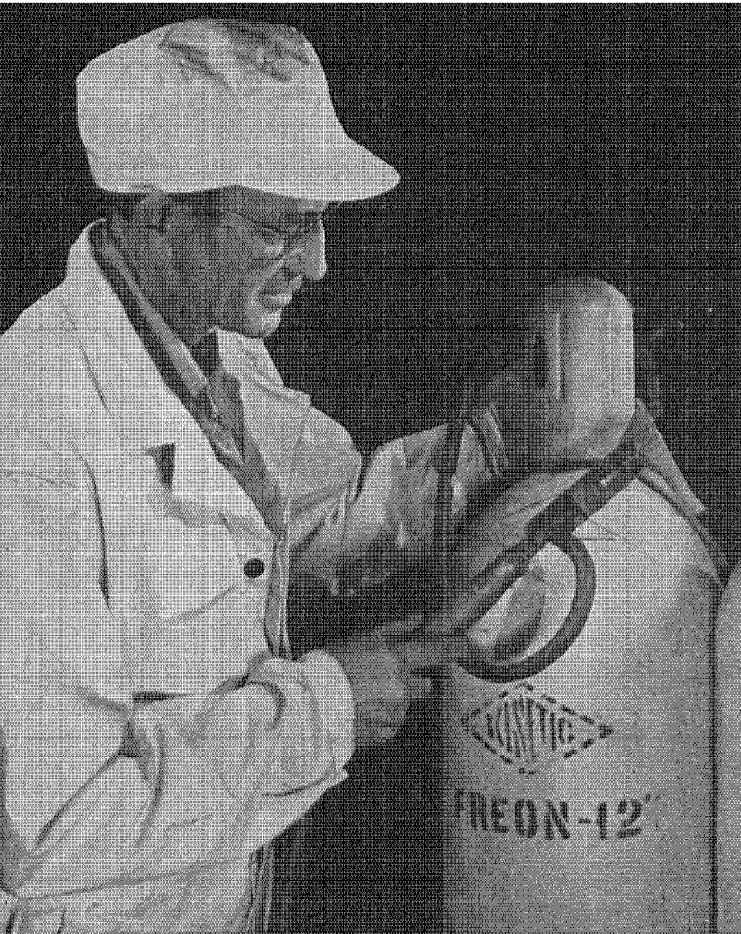
Checking a cylinder of "Freon" for leakage with a halide lamp prior to shipment from the plant.
