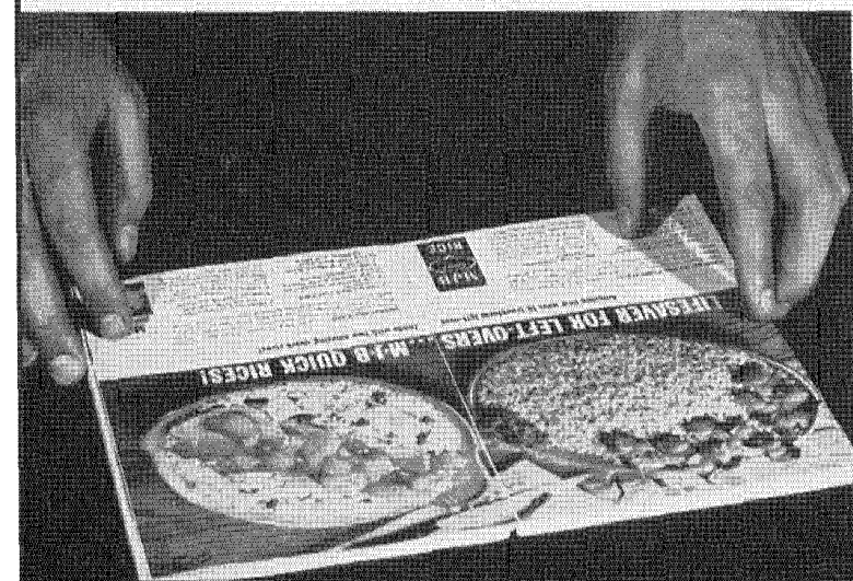
Magnified photo of end of a Digest hanging by its covers shows how film of hot-melt adhesive (arrow) welds pages, cover together.
