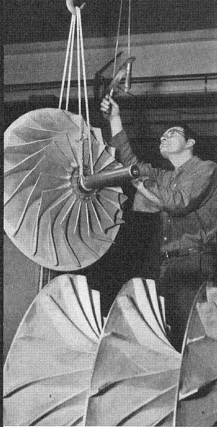
Two jobs for synthetic fiber slings at Carrier: top, nylon rope moves an impeller wheel for compressor; bottom, nylon webbing carries a 1,500 pound impeller and shaft assembly.
