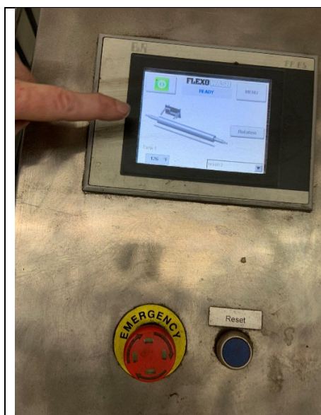
Flexowash (FW-3000-2) with setting options for washing press cylinders. Photograph 11 taken at 12:14pm
