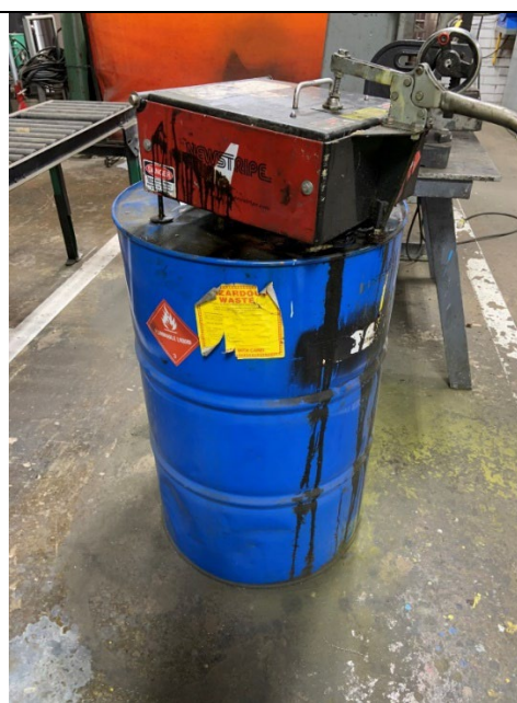
55-gal container with aerosol can liquid remover inside maintenance room. Photograph 32 taken at 1:05pm
