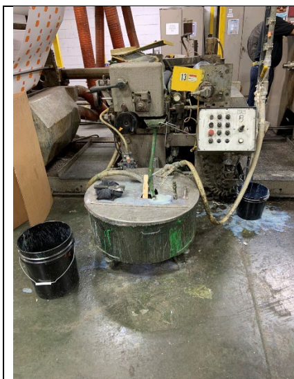
Press 7272 with dry coating in bucket and on floor. Photograph 3 taken at 11:14am
