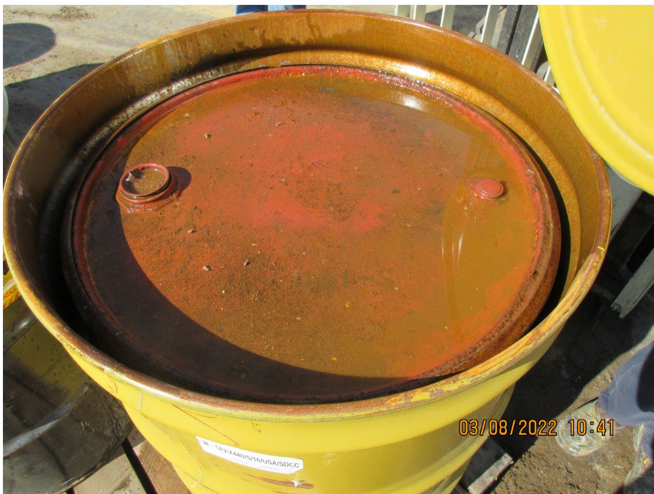
Photo 4 – Drum floating in water within overpack container in Row 32 of Unit 217 shown in Photo 3.
