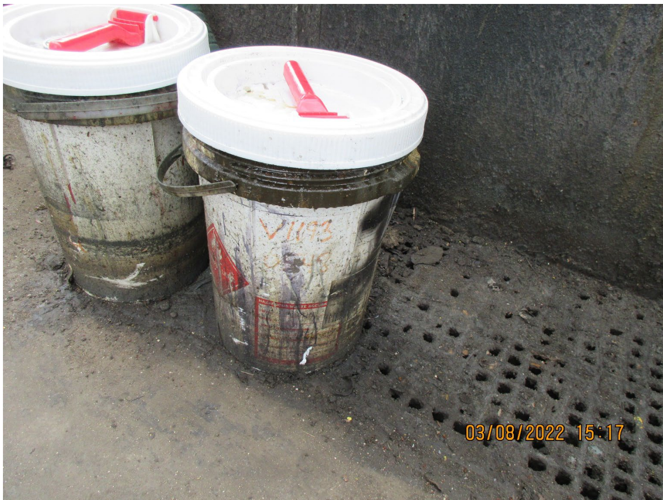
Photo 6 – Five-gallon hazardous waste containers in SAA in the area of permitted tanks in Unit 208
