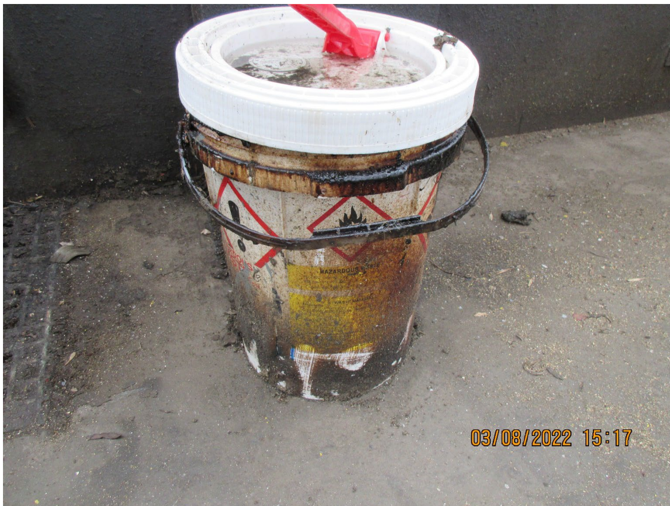
Photo 7 – Five-gallon hazardous waste container in SAA in the area of permitted tanks in Unit 208
