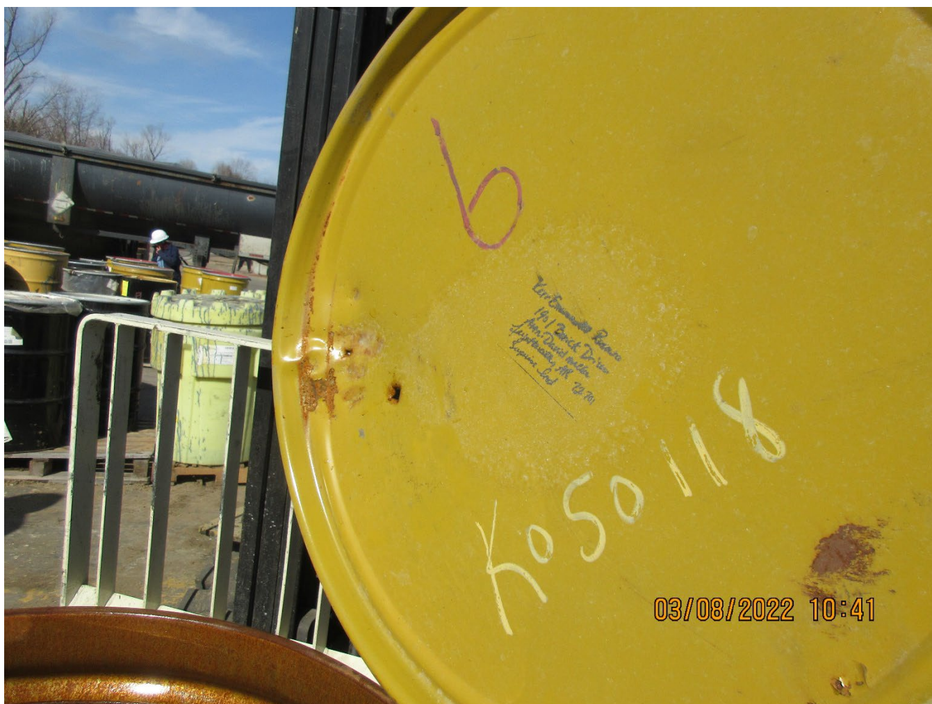
Photo 3 – Hole in lid of overpack container in Row 32 of Unit 217
