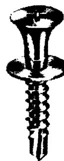
Comp-Rated Screw (patent pending) When driven into the stud to attach metal lath, the screw head projects into the cement plaster forming a structural composite of the joined materials. Self-drilling self-tapping screw is 1-inch long, #8 shank.
