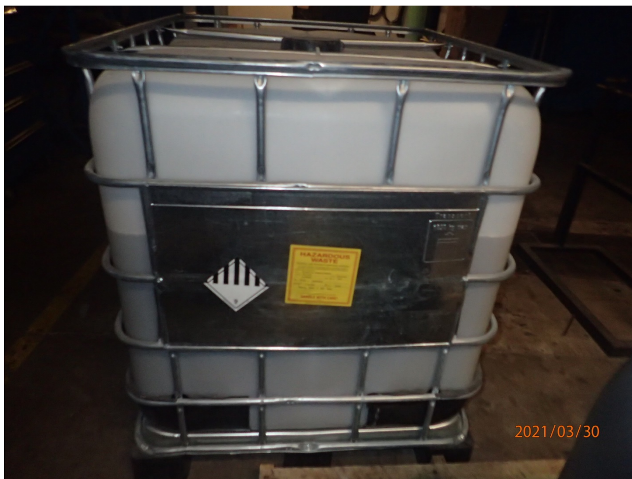
Photo 11: 250-gallon tote labeled “Hazardous Waste – Blasting Media and Paint Waste – D008”. Located at Pen 1 inside Magnolia Plant.
