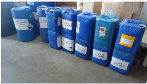
Photo #43 – Hazardous plating waste containers in the wastewater treatment system area.
