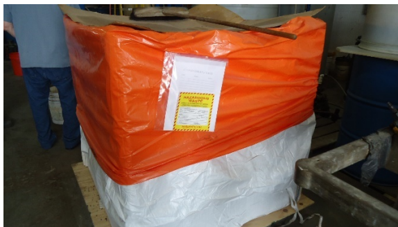
Photo #49 – F006 filter cake sludge stored in a 250-gallon tote.
