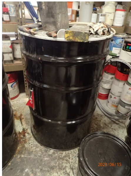
Photo #2 – Open and unlabeled satellite accumulation container in the Chemical Lab.
