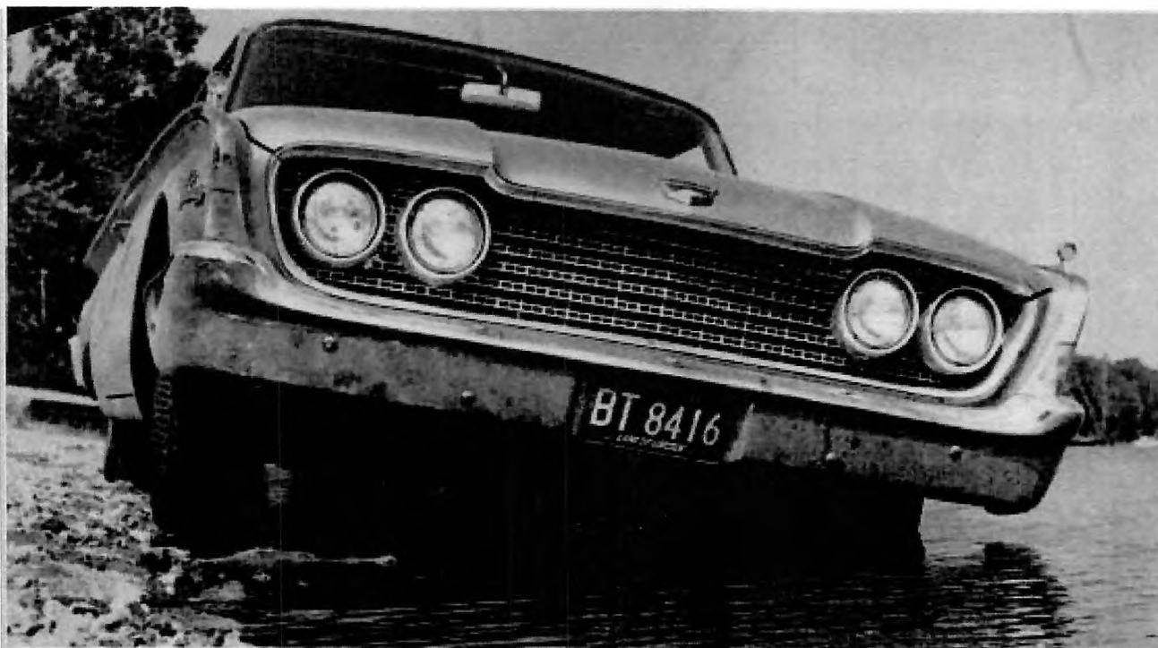
WET-BRAKE-STOPPING power test was made by driving car into nearby lake to soak the drum and linings
