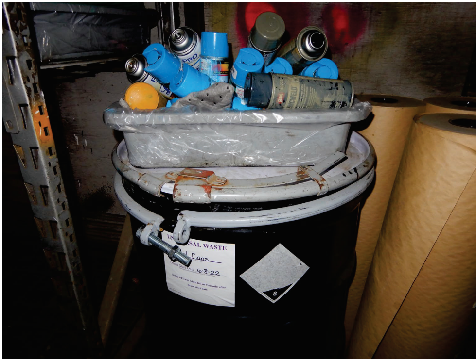
Photo 4 (DSCN0051.JPG): Universal waste aerosol cans in open and unlabeled tray
