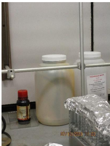
Photo 11: In the Chemistry Lab, in workstation B316, the inspectors observed one gallon-sized closed container with material inside but no label (Photo 11).
