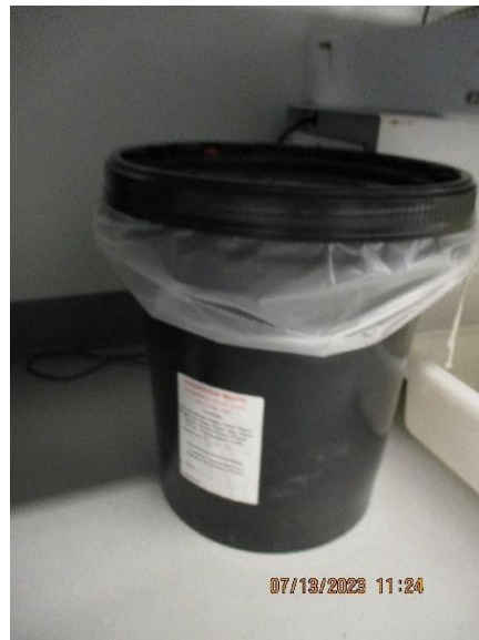
Photo 14: In the SFC Chromatography area, a 5-gallon SAA for each instrument. Each container was closed, labeled with the words “hazardous waste” and labeled toxic to indicate the hazard of the contents.
