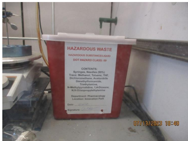
Photo 10: In the Chemistry Lab, each hood has a one-gallon container of waste syringes and needles. The containers were labeled "DOT Hazard Class:09".
