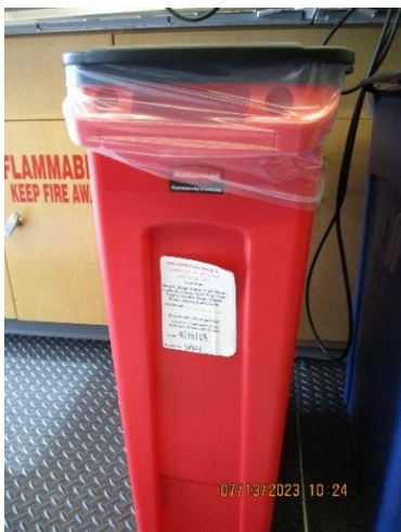
Photo 9: In the Chemistry Lab, each bay also has a 20-gallon red container for flammable, toxic solids.
