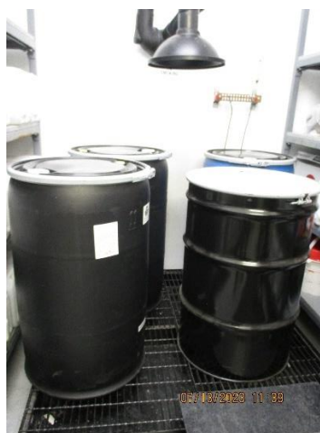
Photo 18: 55-gallon hazardous waste containers in the CAA. Containers are labeled, dated, closed, and marked with the indication of the hazard of the contents.
