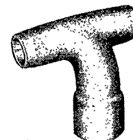
No. 1365, Short Type Wash Tray Sink Tee Copper to Copper to Inside I. P. S. Made in \frac{1}{2} -inch size only. This Tee is a short radius fitting that can be installed in a very small space. The run has solder-joint openings; the outlet has a female iron pipe thread.
