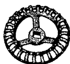
Style F Wheel, Malleable Iron Non-Heat, Round Pattern, Square Hole Widely used on smaller size Brass, Iron and Steel Valves (Globe, Angle, and Cross, and Non-Rising or Rising Stem but not O.S. & Y. Gate). Larger sizes of such valves are fitted with Style D Wheels.
