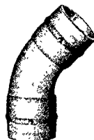
No. 1384, Wrought Tube 45° Elbow Copper to Copper Straight sizes, \frac{3}{8} to 2-inch
