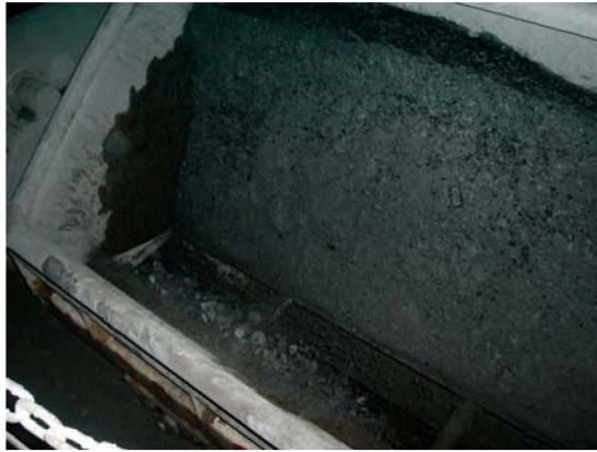
(a) Inside of Hopper before liners were installed
