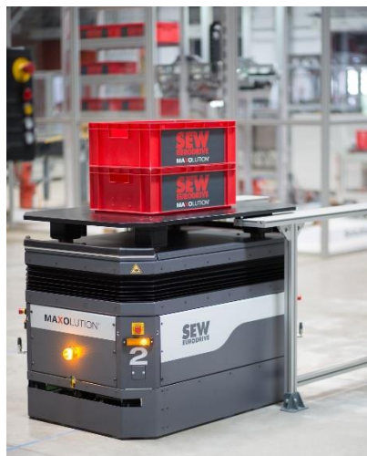
Figure 8 Automated guided vehicle with oscillating drive wheels © SEW-EURODRIVE GmbH & Co KG
