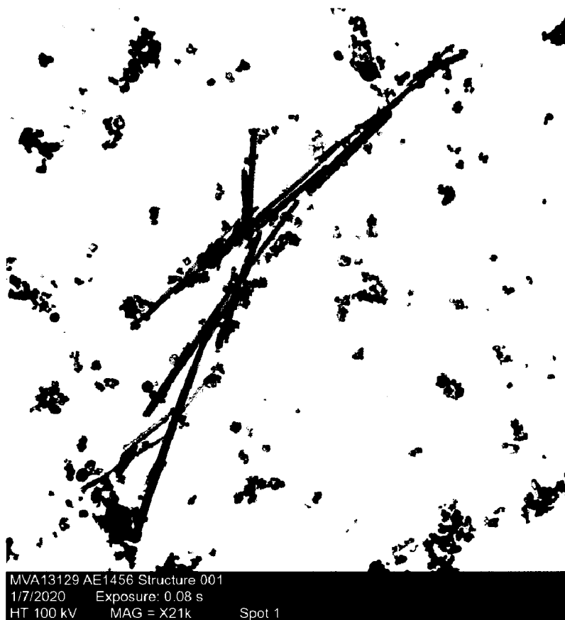
Figure 38. TEM image (above) and EDS spectrum (below) of a chrysotile fiber bundle from air sample AE1456 (Test B – Pump #01).
