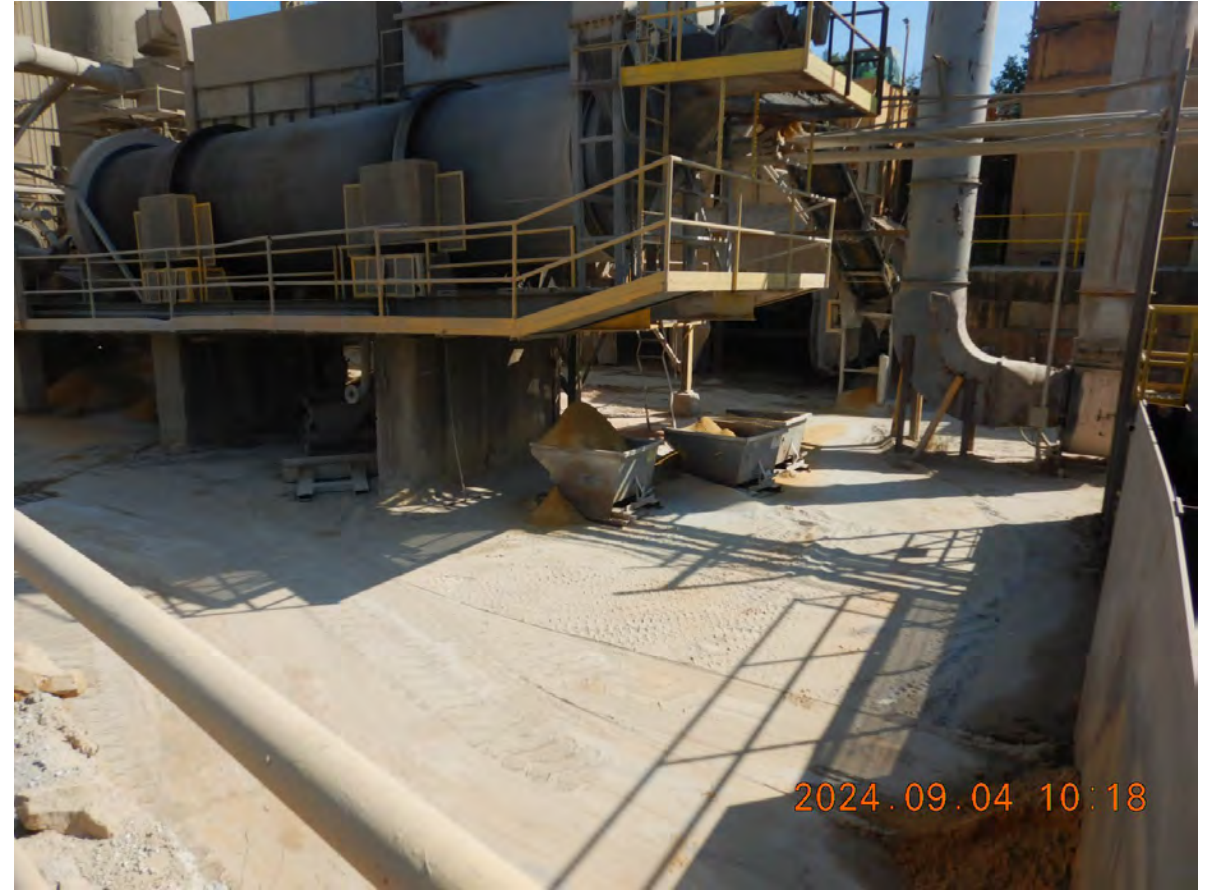
DSCN3739 – Central area of Site near silos; material collected to be recycled; material overflowing dust collectors
