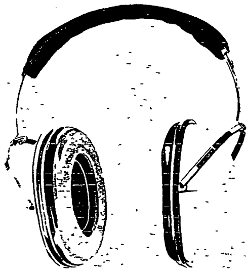
FIG 38-8c - Fluid-filled cushion-type muff
