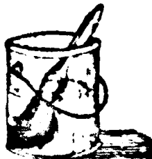
Fig. 45. The WRONG WAY to store brushes.
