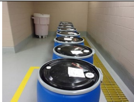
Figure 16: 10:39 AM Flammables Storage Eight of twenty-three 55-gal containers with hazardous waste label, accumulation start date, and an indication of the hazards of the contents.
