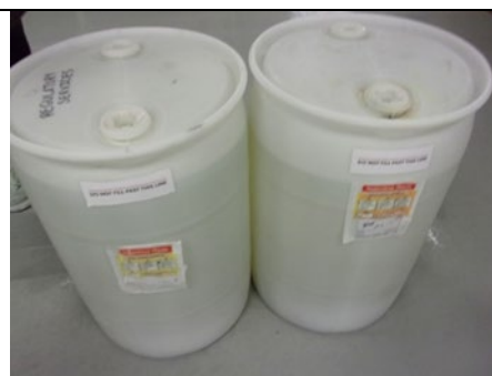
Figure 10: 10:27 AM Metals Storage Two of six 55-gallon containers with hazardous waste label, accumulation start date, and indication of the hazards of the contents.
