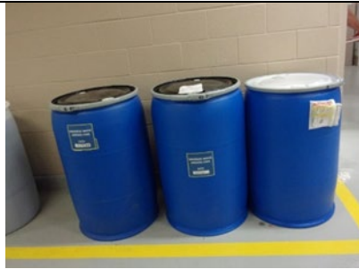
Figure 19: 10:42 AM Flammables Storage Two (2) 55-gal containers of universal waste aerosol cans and one of twenty-three 55-gallon containers with hazardous waste label, accumulation start date, and no proper indication of the hazards of the contents.
