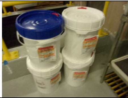
Figure 6: 10:26 AM Metals Storage Four (4) 5-gallon containers with hazardous waste label, accumulation start date, and indication of the hazards of the contents.
