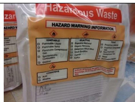
Figure 34: 12:06 PM Chemical Engineering Building: Room 770 One of two bag containers observed in SAA. No indication of the hazards of the contents.
