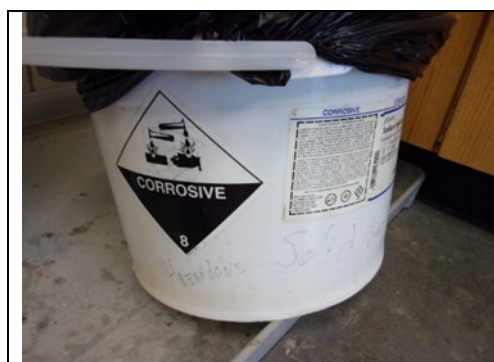
Figure 33: 11:33 AM CP 239, 243, and 245 (Photo 2 of 2) 3-gallon SAA container observed with a corrosive indication of the hazards of the contents.
