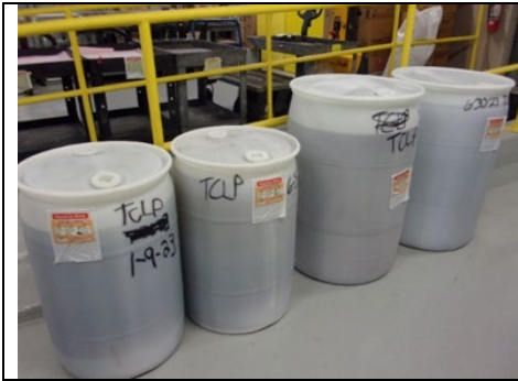
Figure 5: 10:26 AM Metals Storage Two of six 55-gallon containers and two 35-gallon containers with hazardous waste label, accumulation start date, and indication of the hazards of the contents.
