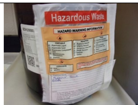
Figure 36: 12:07 PM Chemical Engineering Building: Room 770 One 2.5-liter container observed in SAA. No indication of the hazards of the contents.
