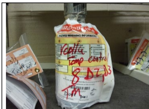
Figure 25: 10:50 AM Reactives Storage One 500-milliliter container with hazardous waste label, accumulation start date, and an indication of the hazards of the contents.
