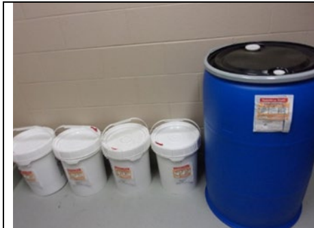
Figure 15: 10:34 AM Flammables Storage Four (4) 5-gallon containers and one of twenty-three 55-gallon containers with hazardous waste label, accumulation start date, and an indication of the hazards of the contents.
