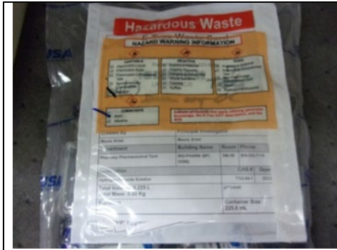
Figure 13: 10:32 AM Oxidizer Storage One 1-liter container with hazardous waste label, accumulation start date, and no proper indication of the hazards of the contents.
