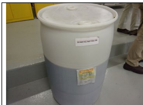
Figure 9: 10:27 AM Metals Storage Four of six 55-gallon containers with hazardous waste label, accumulation start date, and indication of the hazards of the contents.
