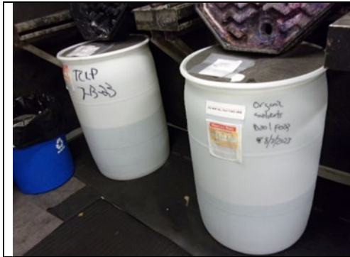
Figure 21: 10:46 AM Bulking Two of three 55-gal containers observed. Containers included a hazardous waste label, accumulation start date, and an indication of the hazards of the contents.
