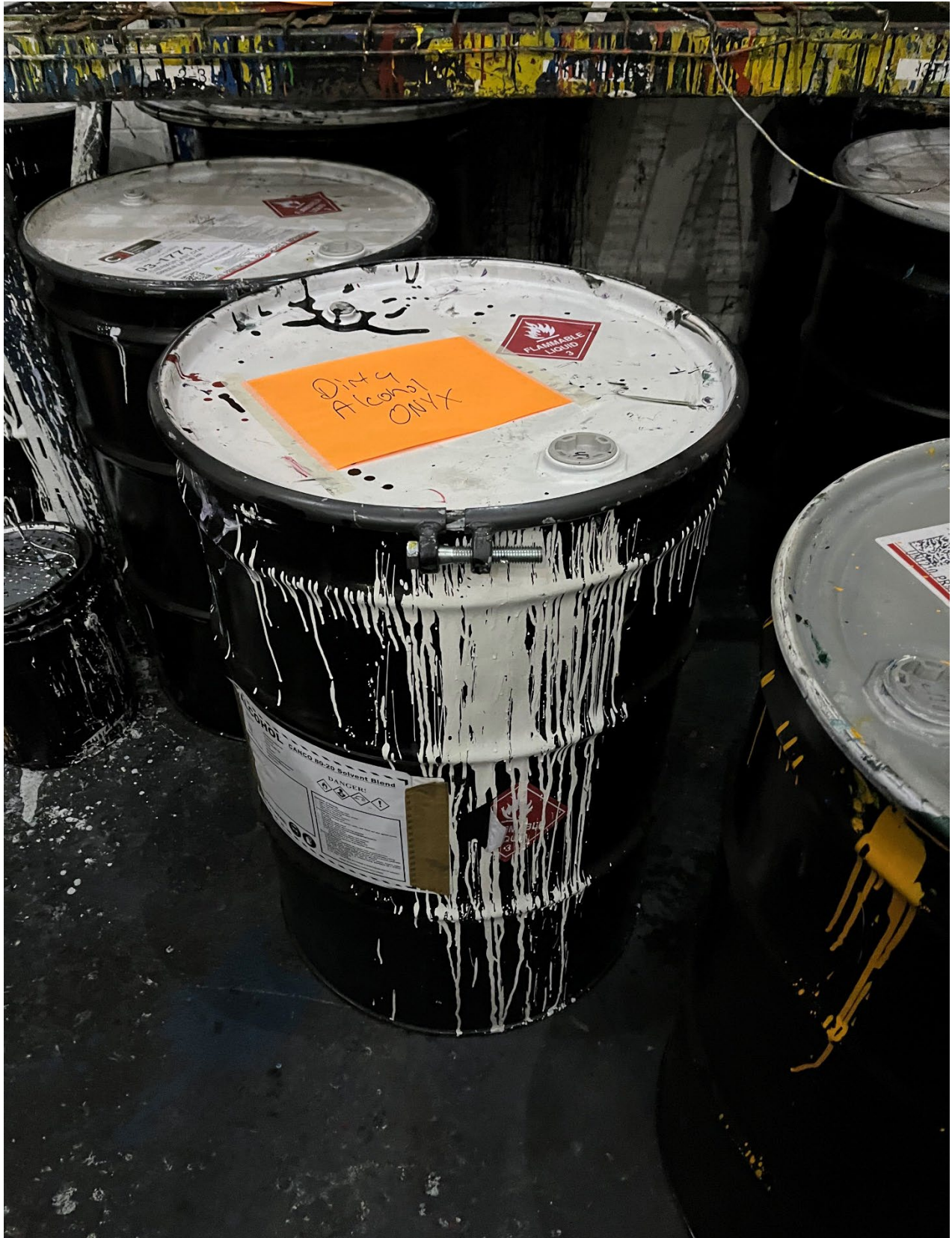
Photo #3: A second drum of waste alcohols in the Ink Room with no hazardous waste label.
