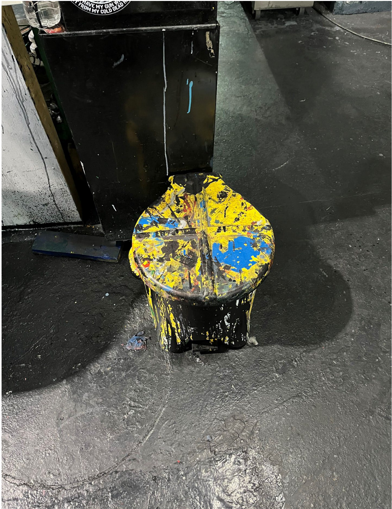
Photo #9: A 5-gallon satellite container of used gloves (no hazardous waste label).
