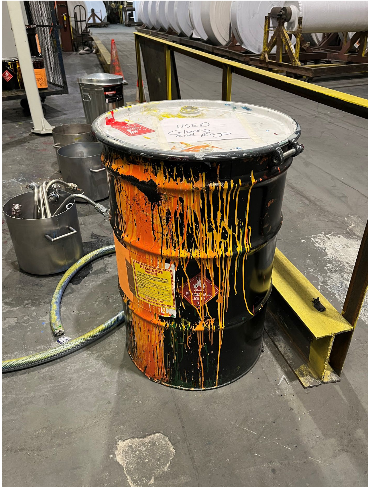
Photo #8: The above drum after a hazardous waste label was affixed.
