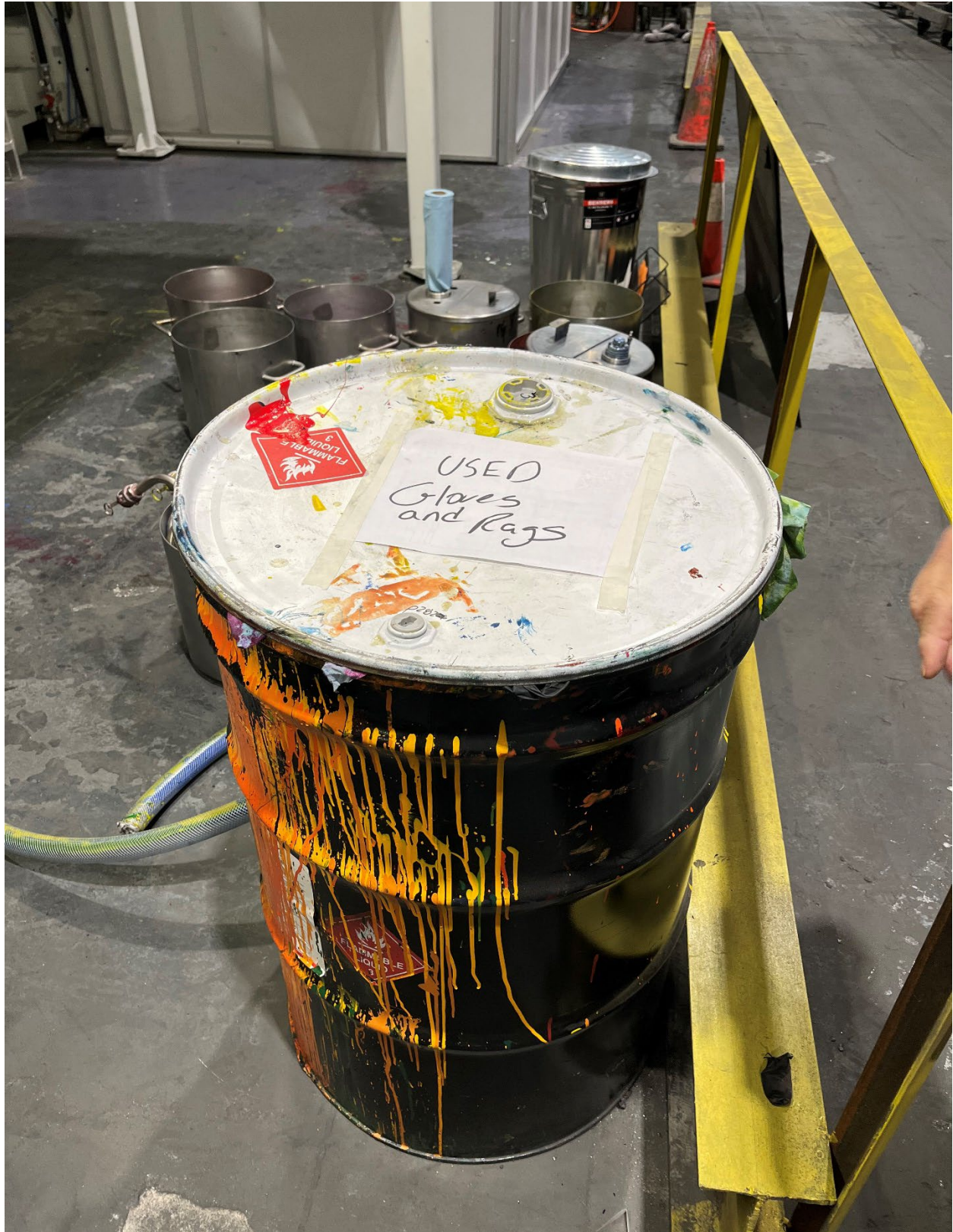
Photo #7: A 55-gallon satellite container of used rags and gloves (no hazardous waste label).
