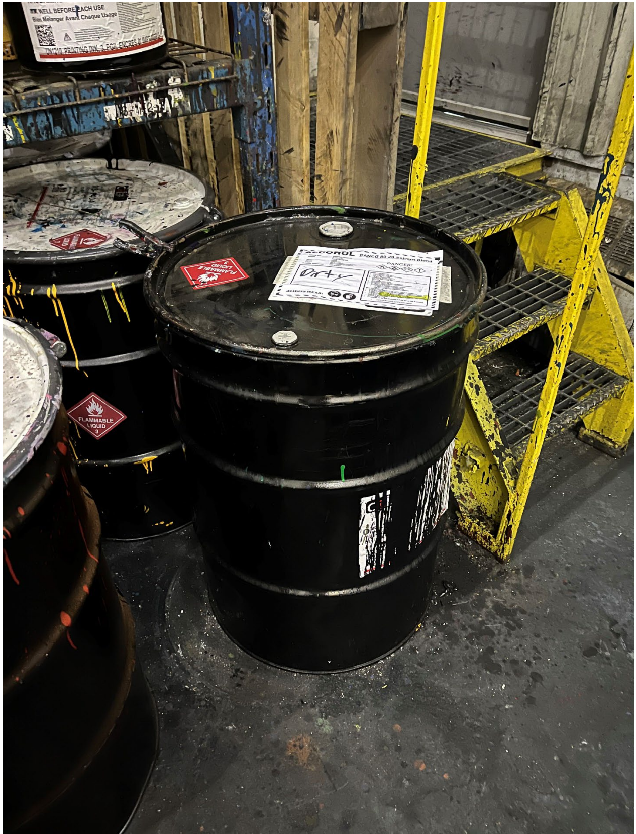
Photo #1: A 55-gallon drum of waste alcohols in the Ink Room with no hazardous waste label.
