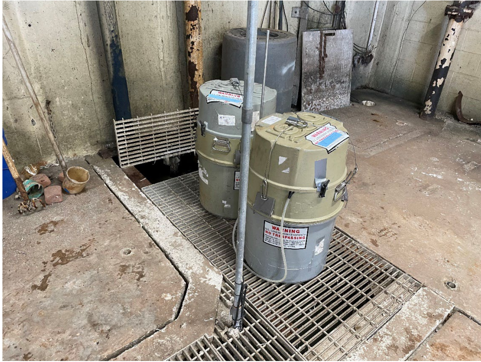
Photo #1. 6-Hour & 24-Hour composite samples were collected from the influent sample point.
