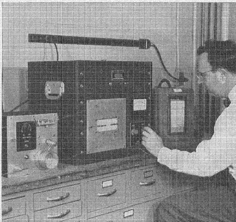
Measuring variations in yarn so slight that conventional equipment can't detect them. More uniform yarn is goal.
