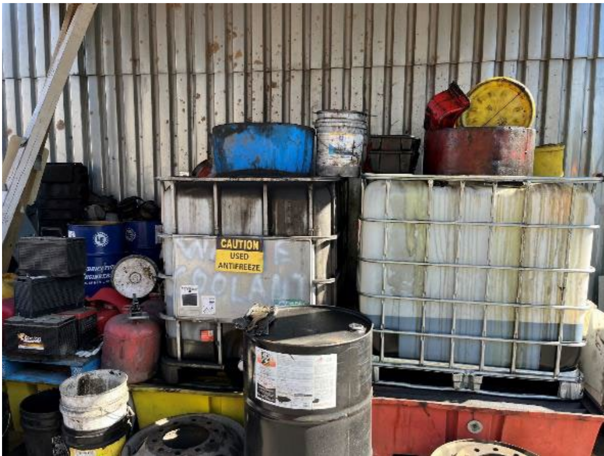
View of used antifreeze, used oil and used batteries, stored adjacent to the maintenance shop. The used batteries are not labeled. {Photograph 29, Attachment 1}
