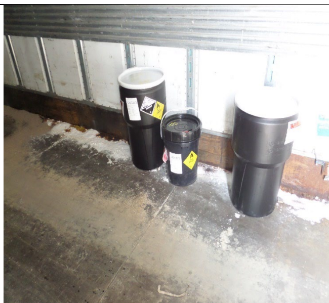
Warehouse. Maumee Express, Inc. (MXI) Trailer #5224. The inspector observed three containers accumulating hazardous waste near the back of the trailer. The inspector also observed a spill of a possible corrosive liquid on the floor of the trailer. The facility was in the process of responding to the spill by neutralizing it and conducting a waste determination. Photograph 6 taken at 11:49 a.m.
