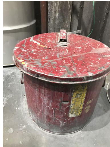
Photo 12: One (1) 5-gallon container of solvent rags, container was closed, no label, no accumulation start date.
