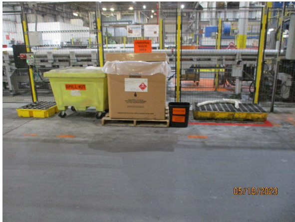
Photo 7: Universal Waste Storage Area 2 for used aerosol cans. Container was labeled “universal waste”, with a start accumulation date, but slightly open.
