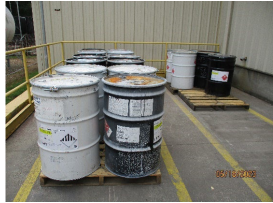
Photo 18: (18) 55-gallon drums of hazardous waste in the CAA for drum waste.
