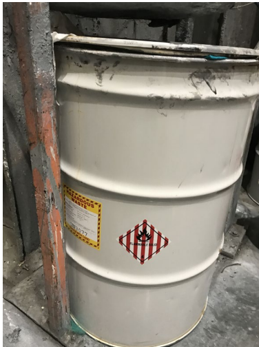
Photo 11: One (1) 55-gallon drum of paint debris solids (filters), drum is slightly open, labeled “Hazardous Waste”, and with an indication of hazard.
