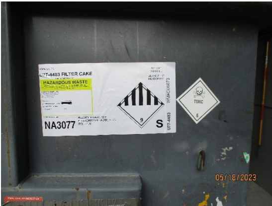
Photo 21: New toxic placard added to roll off container of filter cake since Class 9 placard does not indicate the hazard content.
