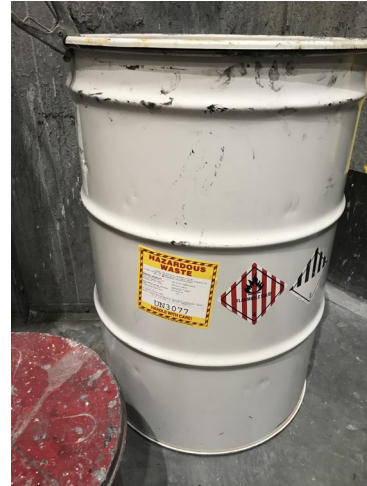
Photo 10: One (1) 55-gallon drum of paint debris solids (filters), the drum was closed, labeled “Hazardous Waste” and with an indication of hazard.
