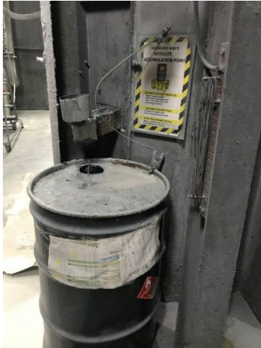
Photo 9: 55-gallon drum of paint sludge/ still bottom actively collecting paint sludge. Container is labeled “Hazardous Waste” with an indication of hazard.
