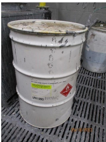
Photo 15: One (1) 55-gallon drum of waste sludge (still bottom), labeled “Hazardous Waste”, marked with an indication of hazard, and not securely closed with a drum ring.
